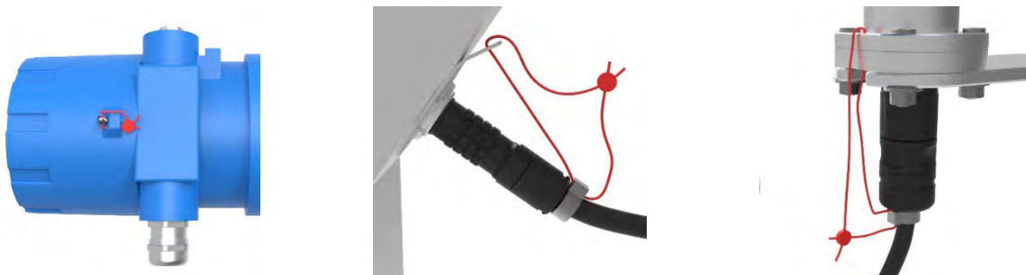
Fig. 12: Seals of the electronics housing and the connector
